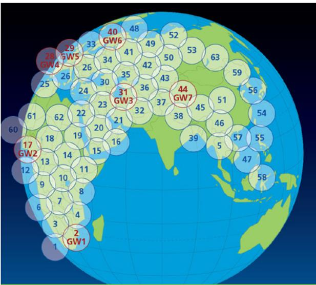
Fig. 1: IS-33e Ku-band User & Gateway Beams
